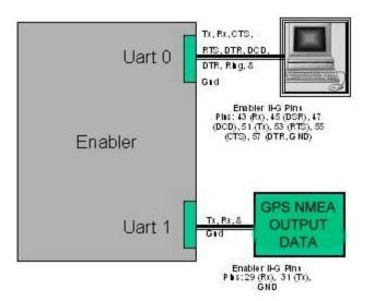
Figure 14 Enabler II-G A-GPS Module Serial Interface with Dedicated Serial Port and GPS Port
